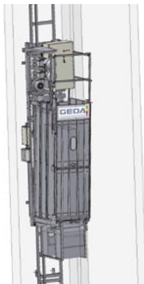
Picture Shows a GA drawing of a GEDA SH in a 100m Pylon in Belgrade. The challenge in the whole design was that we just had a shaft width of 1,2m and the Pylon has a inclination of 2,36 degrees
